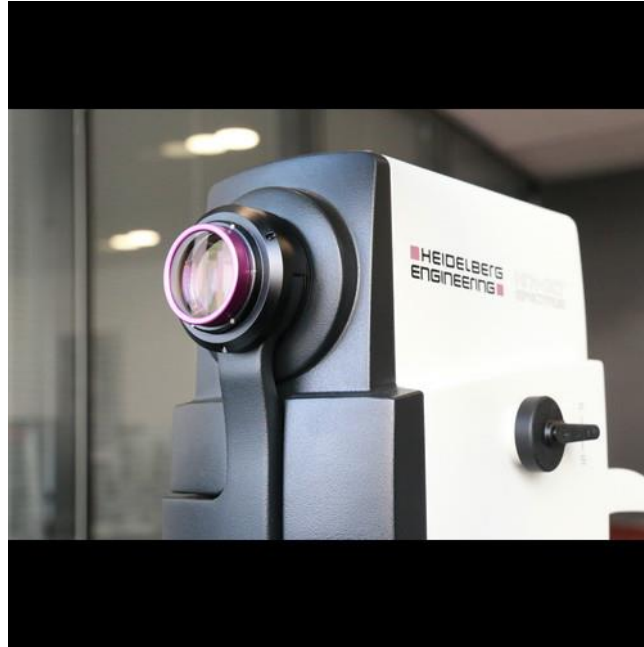
Figure 3 Heidelberg Engineering's SPECTRALIS High Magnification Module Top: High Magnification Lens (hot pink) Affixed to the SPECTRALIS Camera Head Bottom: High Magnification Images
